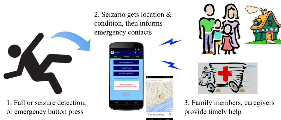
Figure 4 Seizario smartphone app for immediate geographical localisation and emergency response notification.
